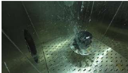
Length measurement sensor 48-hour rain-proof test
