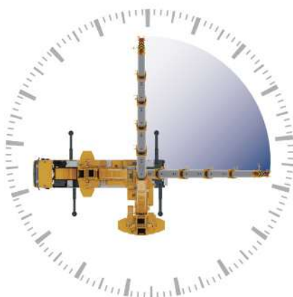
The minimum stable slewing speed is 0.1° /s
