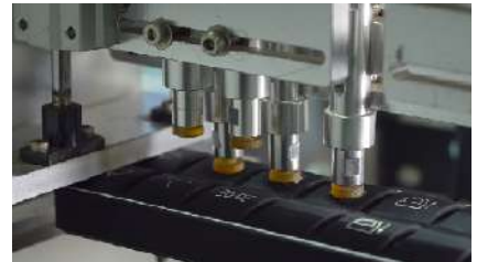
Panel buttons 1.2 million times reliability test
